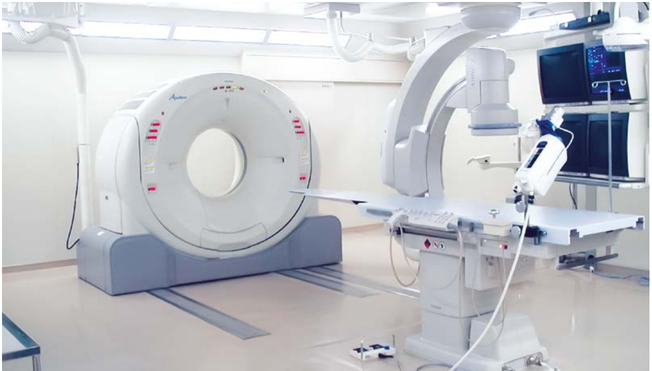
Figure 7: The ceiling C-arm can park perpendicular to the table and CT gantry. This unique design doesn't disturb patient approach from both right and left side of the patient
