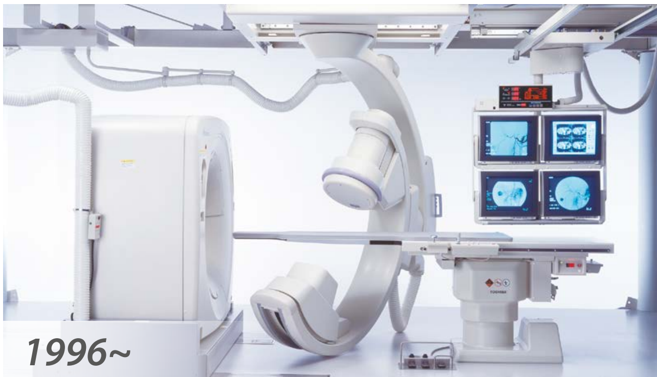
figure 5: The Angio CT system produced in 1996. The CT gantry is now movable on the floor rail. The basic design of the well-known Angio CT system was invented at this time.
