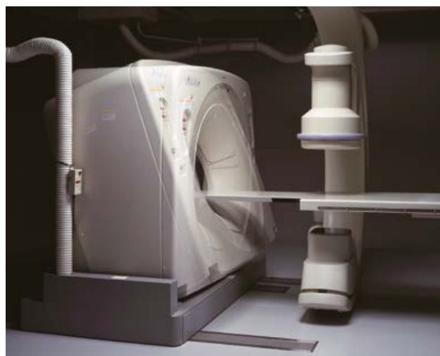
The CT base can move on the floor to realize the helical scan. This unique concept was born by Toshiba/Canon in 1996.
